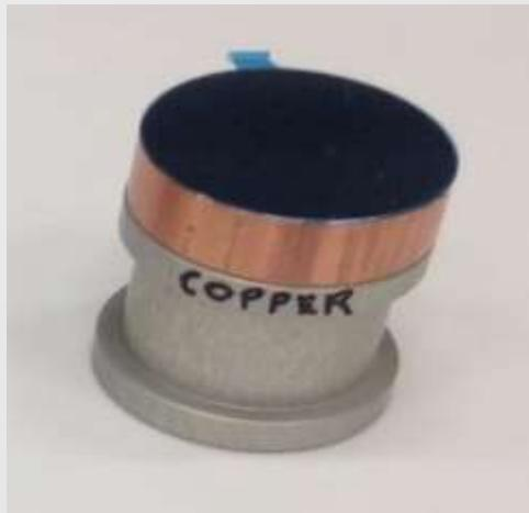
Copper is a soft and ductile metal which exhibits a relatively plastic response and therefore work hardens as a function of deformation. Exposure of its surface to ambient air will produce a native cuprous oxide layer ( $Cu_2O$ ) which may have a thickness of 100 nm or more.
